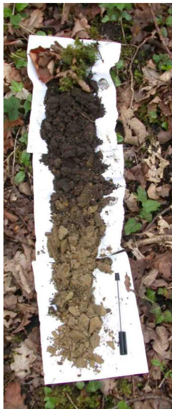
Figure 3. A soil profile derived with a Dutch soil auger. Samples are taken from the same core site and laid out in sequence (i.e. topsoil above subsoil above parent material) to ascertain the soil type.
