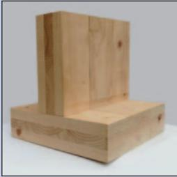
Research carried out by NUIG has established the viability of using grade C16 Irish Sitka spruce to produce structural CLT panels.
